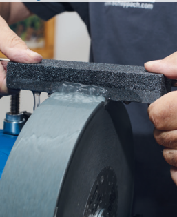
Increased grain size for particularly fine grinding; the other side is perfect for high material removal.
