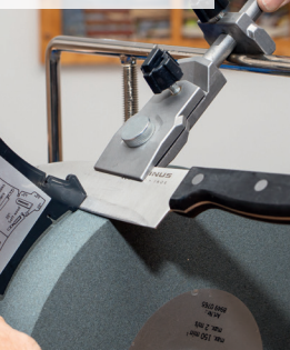
Suitable for knives with a blade length from 40 mm to 200 mm.
