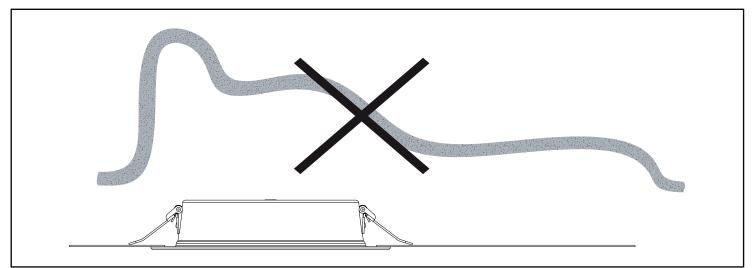
The external flexible cable or cord of this luminaire cannot be replaced; If the cord is damaged, the luminaire shall be destroyed.
