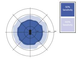
Installation - Ceiling mounted Suggested installation height 2.5-6m
