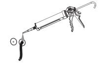
Caulks in knock out holes are tight enough to avoid dust, insects, and especially water from leaking inside.
