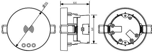
821006001800 - LEDSmart-BLE2-Rc-MW-Sensor
