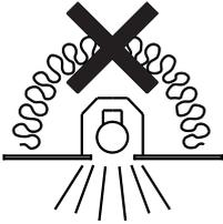
This luminaire is not suitable for covering with thermally insulating materials.
