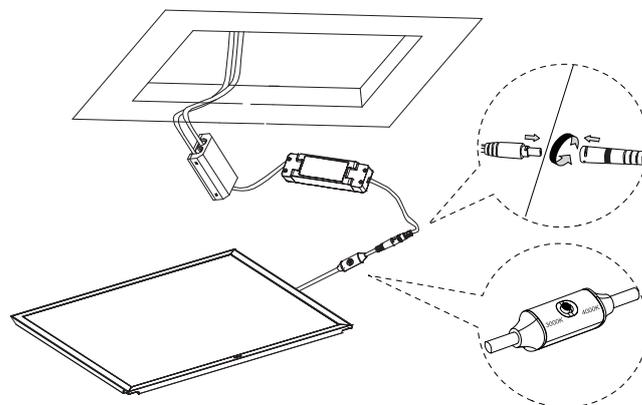
Note: CCT switch is only for double CCT version, the default setting is 4000K.
