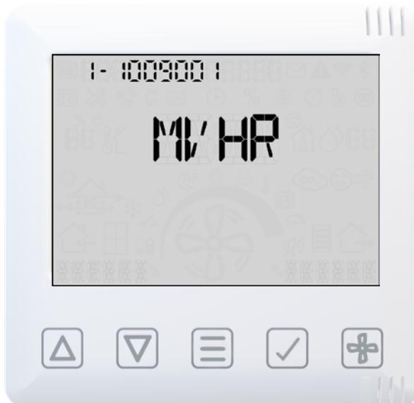
If the primary/additional(secondary) HMI is not paired with mainboard, then MVHR screen will display with cyan LED.
