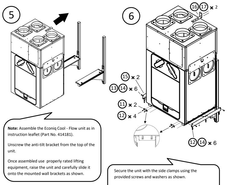
Reattach the anti-tilt bracket other way up and fix to the wall using the wall plugs and screws.
