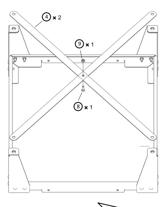
Turn the part assembled kit over and align tie bars (Item 4) with each foot bolt hole as indicated and secure the centre of the tie bars (Item 4) the coach bolts M6 (Item 8), nuts M6 (Item 9) as indicated.
