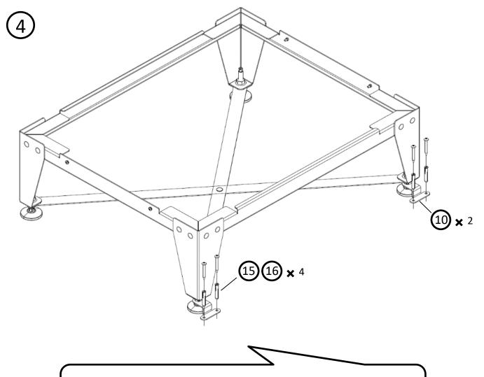
Secure the assembled Floor Mounting Kit on the ground with the foot clamps (Item 10), self tapping screws (Item 15) & wall plugs (Item 16). Use nut positions on each foot to level the floor mount assembly.
