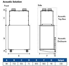
Acoustic Top Box 17kg, Acoustic Enclosure 33kg
