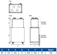
Acoustic Top Box 17kg, Acoustic Enclosure 33kg
