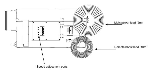
Ports must be covered by label (supplied in accessory pack) to maintain the Moisture Ingress Protection rating.
