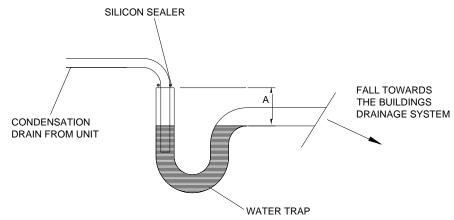
NOTE: INSTALL THE CONDENSATE DRAINAGE TUBING IN ACCORDANCE WITH THE DIAGRAM. ENSURE THE WATER TRAP IS BELOW THE DRAIN ELBOW OUT LET "A"
