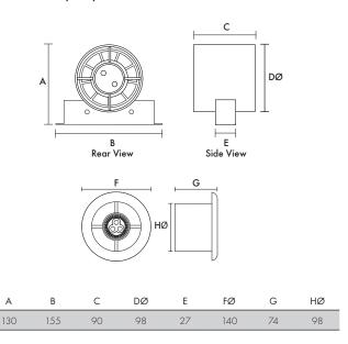
Internal/External Grille Dimensions 140x140mm Fan Transformer (W x H x D) 87 x 87 x 33
