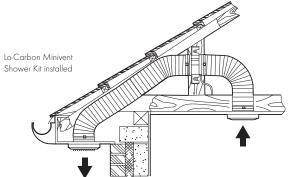
When installed, the fan kit has ample performance to meet the Building Regulations requirements for toilets and bathrooms. The timer version should be used for internal rooms.
