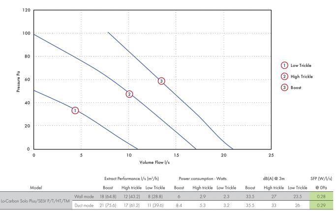
Tested at 240VAC @ 50Hz
