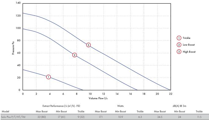
Tested at 240VAC @ 50Hz
