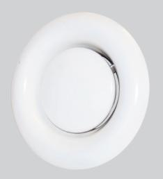
Fire Rated Air Valves are a unique and cost effective fire rated solution where recessed ceiling air valves are to be installed in fire rated floor/ceiling constructions. In a fire situation, the integral intumescent material rapidly expands to seal off the air valve to help maintain the fire resistance rating of the ceiling. This limits the risk of fire and heat spread throughout the building.
