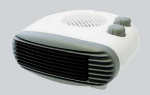
The Vent-Axia Portable Fan Heater is a floor standing heater with three settings, fan only, 1kW and 2kW outputs. Variable thermostat. The unit comes complete with a 13amp plug.
