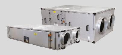
Mini and Midi Models are manufactured with a frameless construction from single skinned Aluzinc panels, internally lined with 90kg/m³ high efficiency acoustic and thermally insulating foam (fire retardant to BS476 Part 7 Class 1 & Part 6 Class O). Aluzinc panels allow for all units to be mounted either internally or externally as standard (IPX4). An optional inlet cowl is available for roof mounting applications if required.
