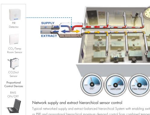
Typical networked supply and extract balanced hierarchical System with enabling switching control (ON/OFF, time clock or PIR) and proportional hierarchical maximum demand control from combined temperature and/or CO<sub>2</sub> sensors.
