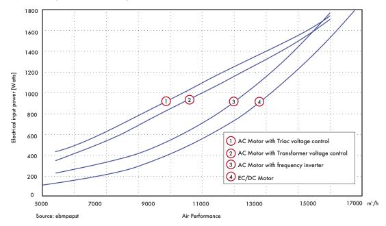
As can be seen from above motor comparisons, the EC/DC motor offers higher efficiencies when compared to AC motors, and also consumes less power under speed control, giving both the highest motor efficiency and lowest power consumption across the speed control range.
